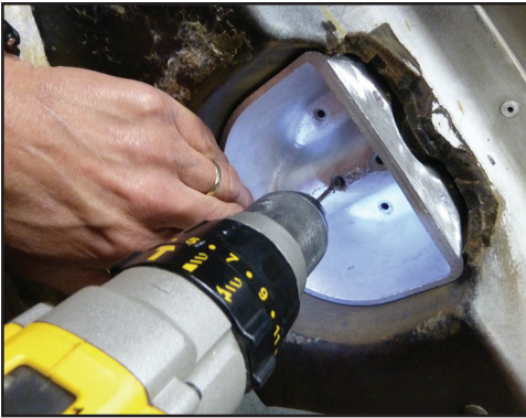
Drill a 1/8" pilot hole into the plastic using the middle plug hole as a guide. Use the correct DRVR or PASS plug, they are different!
