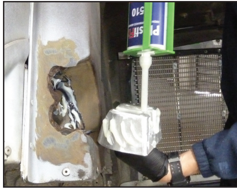
Generously coat the plug and socket with enough PlastiFix adhesive to fill any gaps between the plug and the pocket.
