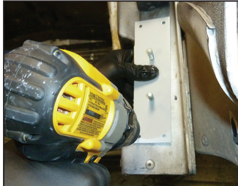
Using two 5/16" x 2" bolts as a guide for the bearing plate, drill the first 3/16" rivet hole into the hood. Note: The plates are identical.
