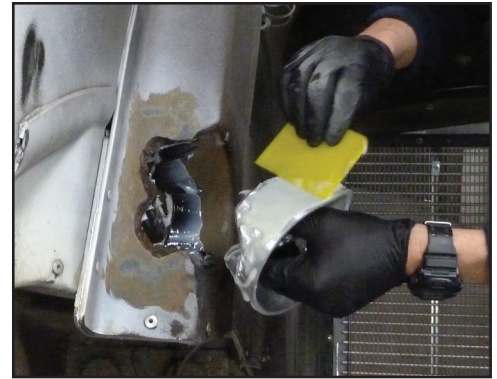
Spread the adhesive evenly over the plug and inside the socket. Working time is about 15 minutes at room temperature.
