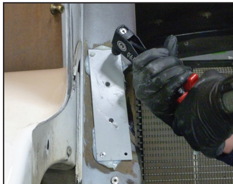
While pushing firmly down on the bearing plate, rivet the plate into place using four 3/16" rivets, one in each corner.
