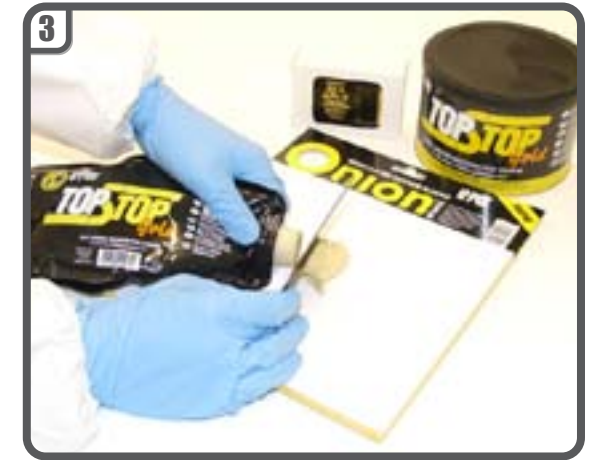
Dispense U-POL Fine Finishing Filler onto Onion Mixing Board .
