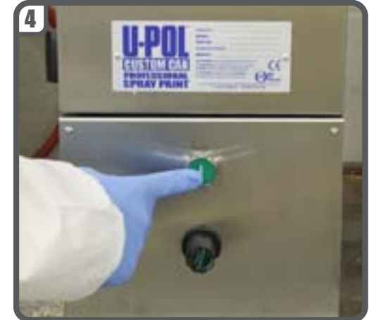
4 Close and lock door. Push green button to activate fill cycle.
