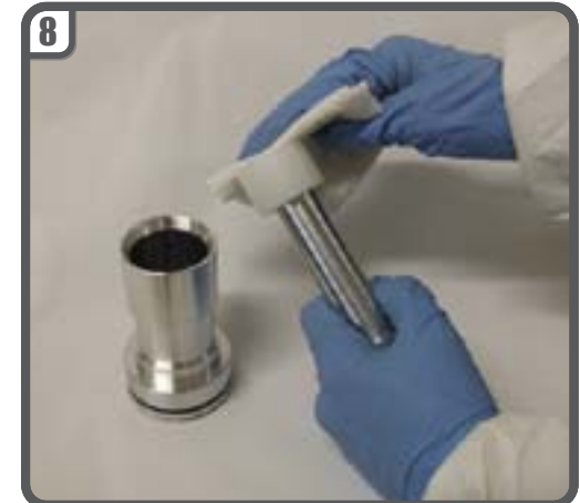
8 Clean piston tip and cup with U-POL Degreaser.
