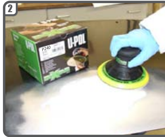
Abrade repair area using palm sander with U-POL P240-500 grit disc . Repeat step 1.
