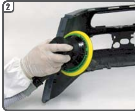
2 Abrade repair area using sander with U-POL P80-120 coarse grit disc . Repeat step 1.
