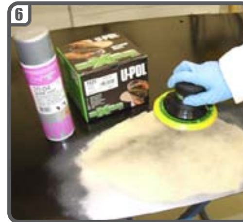
Allow to cure thoroughly and apply thin coat of U-POL Dry Guide Coat S2004/AL . Abrade using U-POL P320-500 grit disc .
