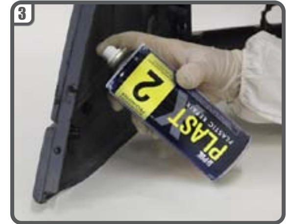
3 Apply one coat of U-POL Plast-X Adhesion Promoter PLAS/2 aerosol and allow to dry for 30 minutes.
