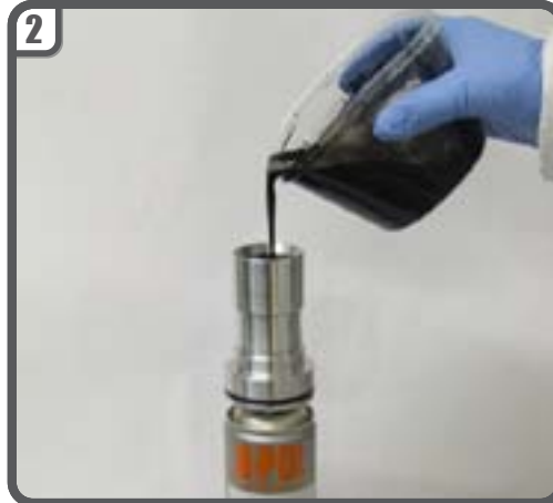
2 Mix paint to manufacturer's recommendations, pour basecoat through U-POL Strainer mesh (size 125µm) directly into Custom Can cup.
