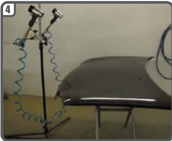
4 Through dry by U-POL DRYFLOW airflow gun (for all waterborne coatings). Direct airflow across paint surface for optimum drying.
