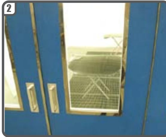
2 Through dry by baking at 60°C in booth (for all coatings except waterborne basecoats).
