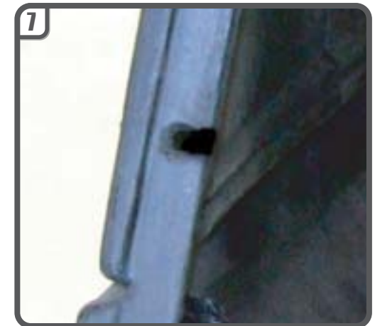
7 Adhesive can be used for re-attaching lugs on bumpers and headlamps, fixing new bolts which have been torn out or applying block of bonding material for drilling and tapping.
