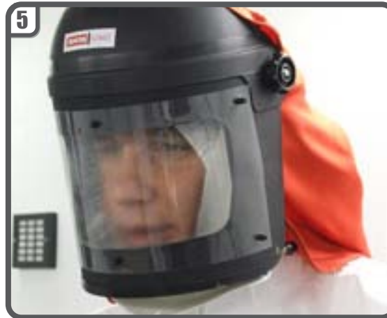
5 Lung and respiratory tract protection with full-face and eye air-fed respirator (when spraying isocyanates).
