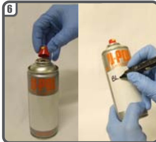
6 Replace aerosol nozzle and lid. Label contents of aerosol with a permanent marker pen. To flush out nozzle, turn aerosol upside down and apply short spray.
