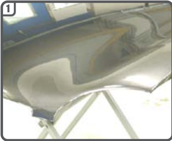
1 Through dry by air (for all coatings).
