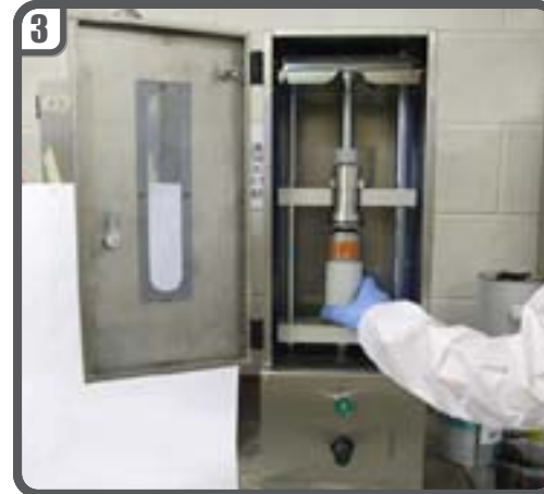
3 Place mounted cup and aerosol into U-POL Custom Can Filling Machine, securing with spring clamp.
