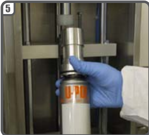
5 Open door, remove mounted cup with aerosol and detach cup from aerosol.
