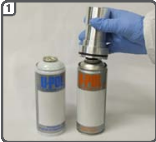
1 Remove lid and nozzle from U-POL Custom Can aerosol. Attach U-POL Custom Can Filling Cup.
