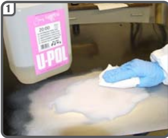
Use lint-free cloth to prepare surface with Water-based S2000 or Solvent-based S2002 Degreaser .
